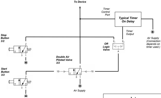
Separate start-stop pushbuttons can be used in conjunction with a double air piloted valve and an "or" logic valve to control a timing circuit if required. A wide selection of types and colours of pushbuttons is available to meet design requirements. The size of the air piloted valve determines the air volume output.
