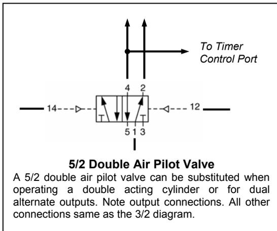
A timing sequence can be established from a momentary pressure signal using an interposing pneumatically operated valve. The most common signal used is from a pushbutton, but inputs from limit switches, foot pedals or other devices can be used to initiate timing. The size of the air piloted valve determines the air volume output.
